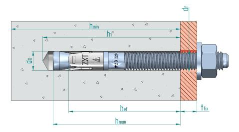
$\begin{array}{ll} d_0 \colon & \text{Nominal diameter of drill bit} \\ d_f \colon & \text{Fixture clearance hole diameter} \\ h_{\text{ef}} \colon & \text{Effective anchorage depth} \end{array}$
